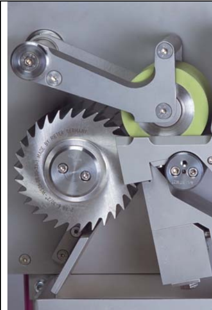
Figure 4. Cutterhead showing beveled surfaces.
