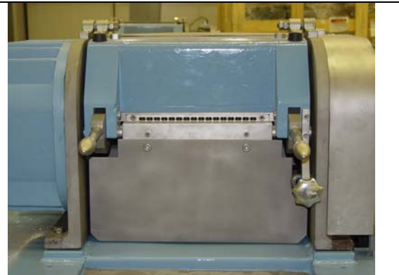
Figure 30. Strand Inlet, now in OSHA compliance.
