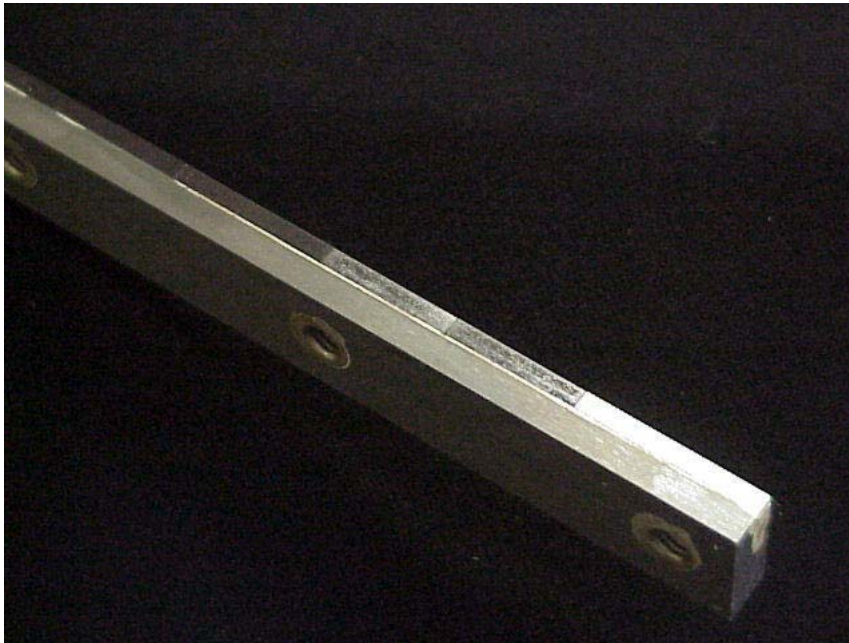
Fig. 10. Bed knife with PCD cutting edge.
