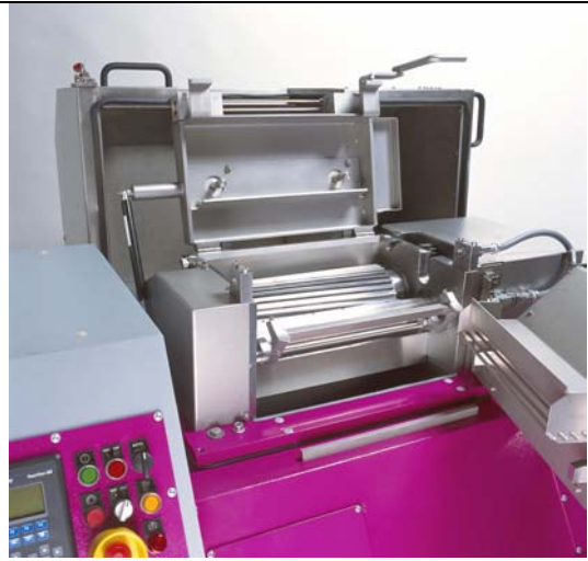
Figure 5. Open cutting chamber showing removal of upper feed roll and swiveling stripper.
