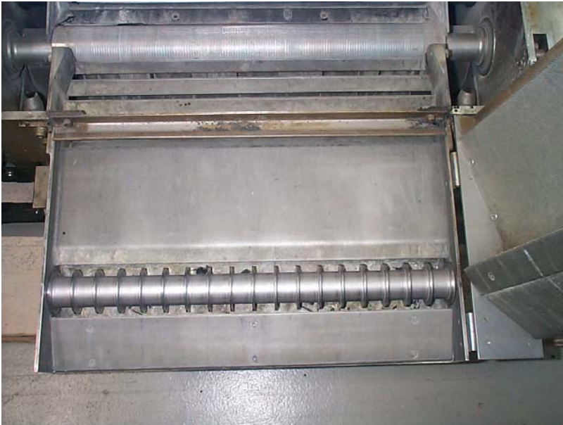
Figure 9. Wear protection type VS 22 after several months of production.
