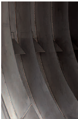
View of helix showing tumbler fins that ensure all surfaces of material are exposed to IR rays.
