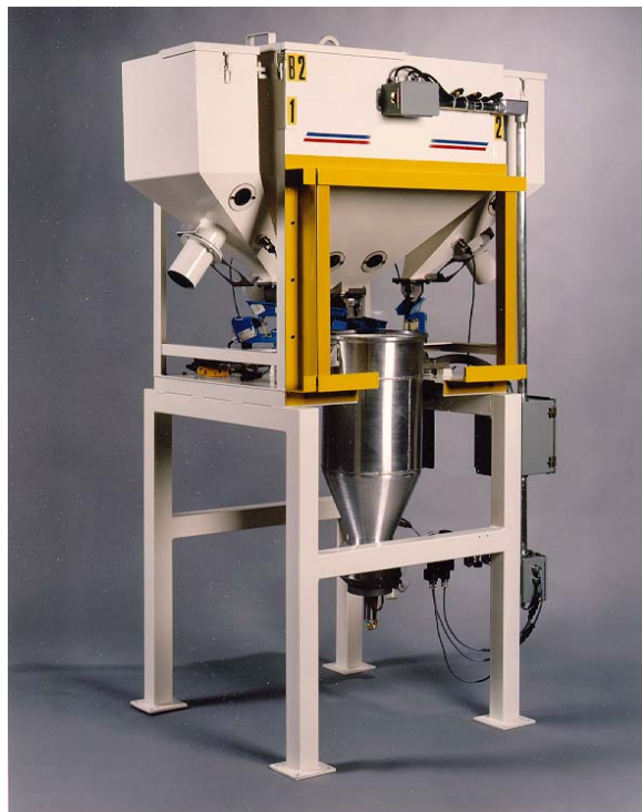
Figure 11. Typical Gain in Weight (Batch Blender) – Multiple feeders sequentially fill a weigh hopper to form a batch. The batch is blended in a downstream or integral mixer.
