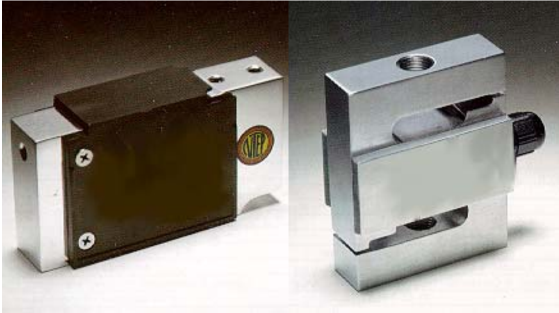
Figure 9. Typical Strain Gauge Load Cells – Shear beam load cell (right) is normally used with weight applied from above on one end and cell fastened to support from bottom at opposite end. An “S” beam load cell is normally used in tension with the cell fastened to support from the top and weight applied from the bottom, however, it can be used in compression with the support and load reversed.
