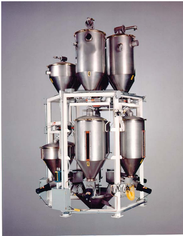
Figure 13. Typical Loss Weight – Target Rate Blender – Individually weighed ingredients are continuously fed at gravimetrically determined proportional rates directly to the downstream process. Static or occasionally continuous dynamic mixers are used if greater blend homogeneity is required. Feeders are usually locked into volumetric feed during refill of weigh hoppers.
