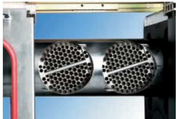
Screen bearing piston moved out for a screen change
