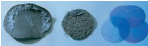
Contaminated and clean screen cloth
