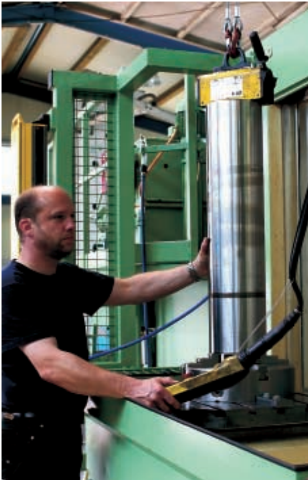
Metal-cutting machining of a screen bearing piston
