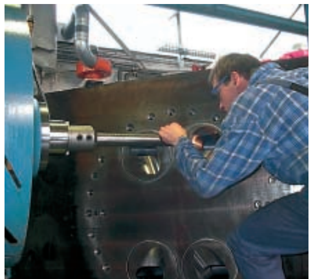
Machining of a housing on the boring machine
