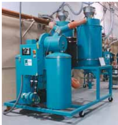
Above: Portable Configuration - Single Dryer and Two Hoppers Mounted on a Single Stand.
