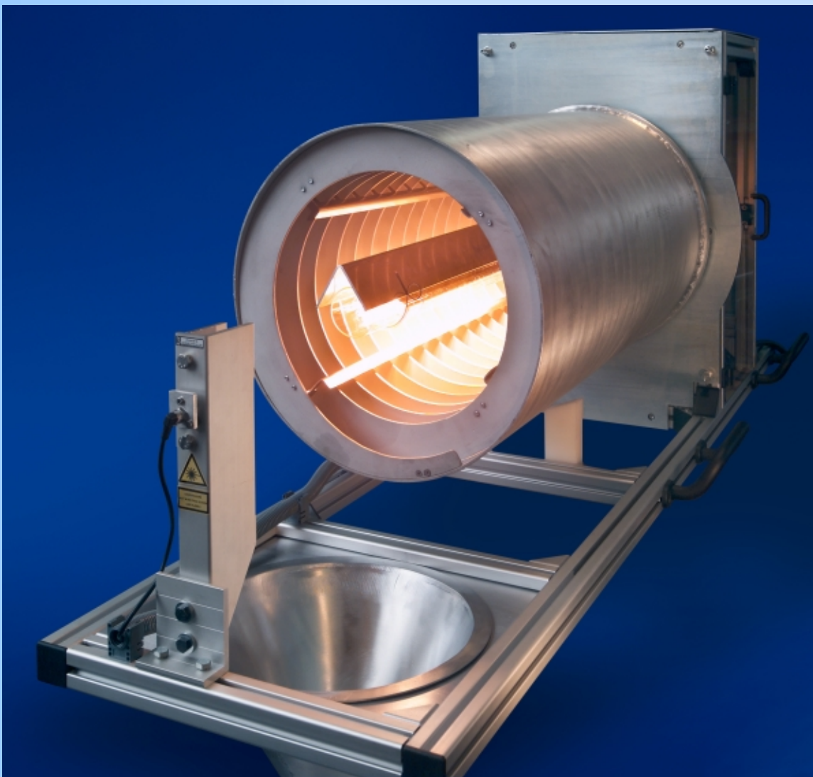
Photo: Infrared Rapid Dryer IR 50/80-6 for small quantities 10-80 kg/h.
