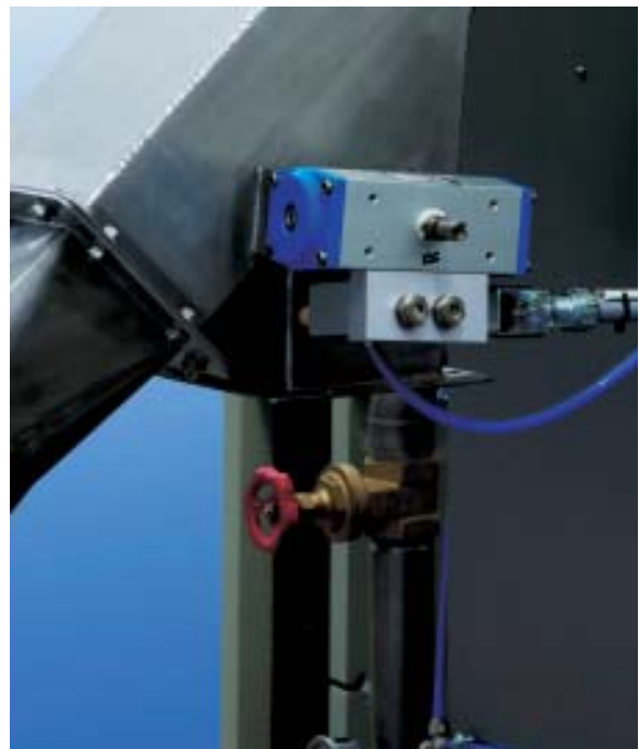
Pellet diverter valve at the dryer outlet
