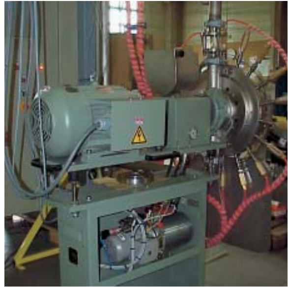
UWG AH 4000 in explosion-proof version (picture taken during inspection for ex-proof certificate)
