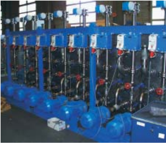
Central water system for feeding of 9 pelletizer systems in a PA6 polymerisation
