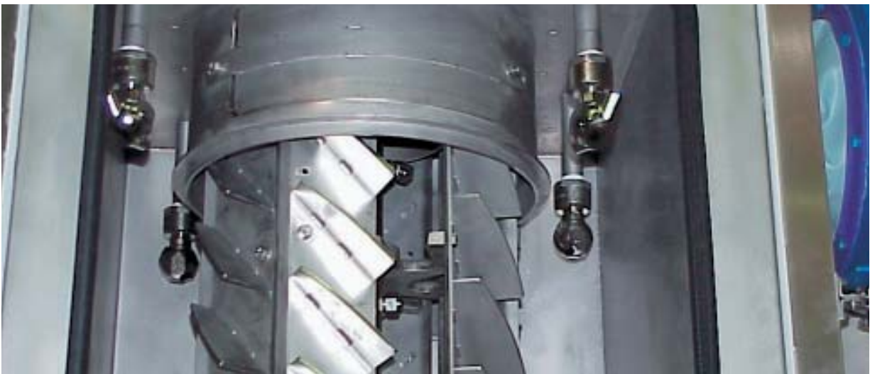
Opti-Line with curved screen and self-cleaning device
