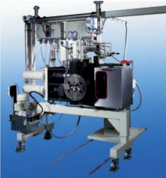
Diverter valve in front of the screen changer and the extruder connection
