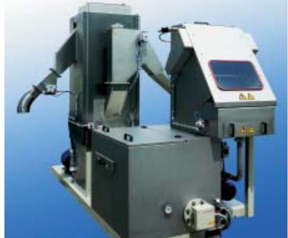
Dryer with self cleaning system
